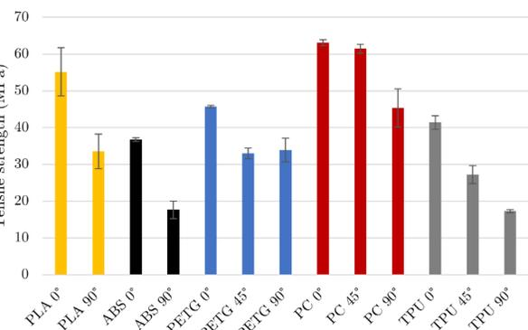
Figure 4 – Tensile strength in different printing orientation for multiple thermoplastic polymeric materials
